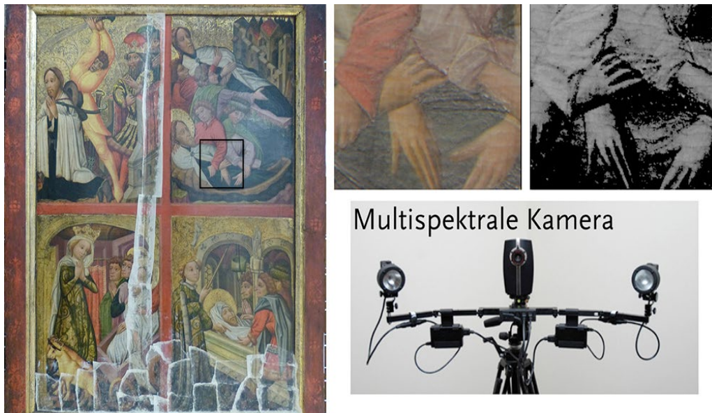
Fig. 6: »Four Events from the Legend of St James the Elder«, Konrad of Freisach, Kunstbibliothek, Staatliche Museen zu Berlin. Photos taken by the multispectral camera in the infrared range revealed a feature that was painted over. The saint's fingers were initially fully exposed but later partly overpainted by work on the sleeve. Enlargements: visual light (left), infrared light (right). Below them is the multispectral camera »Artist«.
