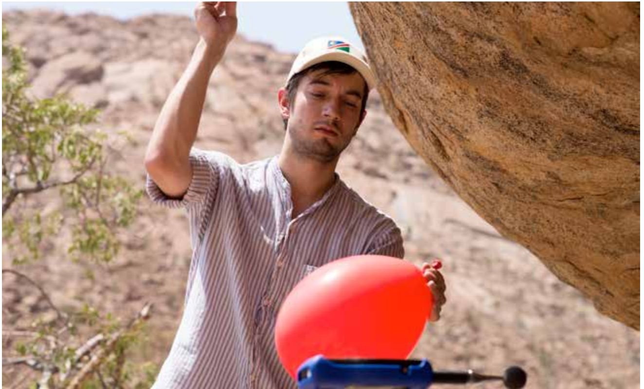
Mobile measurement device: recording the impulse response from an exploding balloon using an audiometer at rock painting sites.
