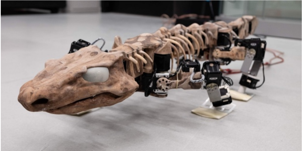
Fig. 5: OroBOT is a physical replica of the stem amniote Orobates pabsti . (Image credits: J. A. Nyakatura | Image Knowledge Gestaltung )
