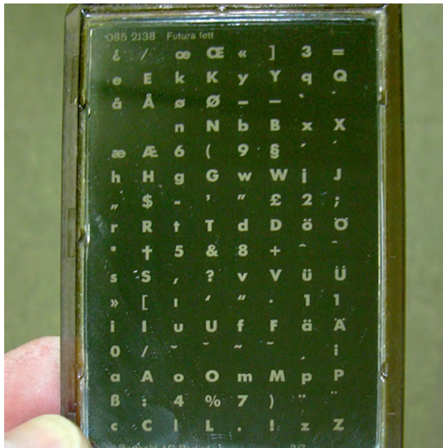
Berthold diatronic matrix plate used in phototypesetting.
