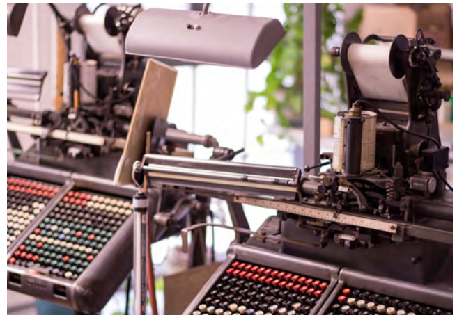
Pushbutton keyboard on a Monotype typesetting machine for producing punched tape, photographed at Offizin Haag-Drugulin Graphischer Betrieb GmbH in Dresden. Photo: Christian Kassung | BWG 2016
