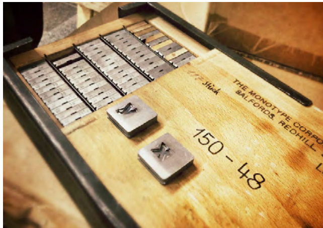
Large type body matrices by Monotype, photographed in the type archives of Offizin Haag-Drugulin Graphischer Betrieb GmbH in Dresden. Photo: Christian Kassung | BWG 2016
